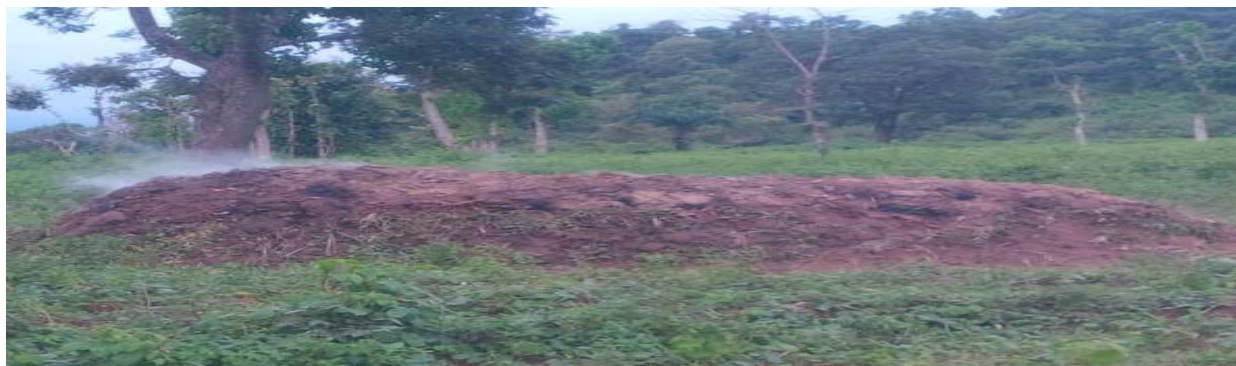
Plate 1. Traditional Earth kiln for Charcoal Production in Kogga (Toro L.G.A of Bauchi State) Source: Field Work, 2017.
